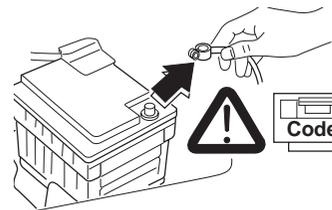
**Disconnect the negative wire from the battery before beginning to install the system and only connect it again after the system has been fitted.**
