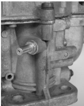
*vacuum-connection is by drilling a 4-mm hole, and cutting M5-thread into the dual choke carburettor (see photo) because these are already prepared for a vacuum nipple. The nipple is supplied with the 123\EVO.*
