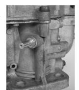
vacuum-connection is by drilling a 4-mm hole, and cutting M5-thread into the dual choke carburettor (see photo) because these are already prepared for a vacuum nipple. The nipple is supplied with the 123\EVO.
