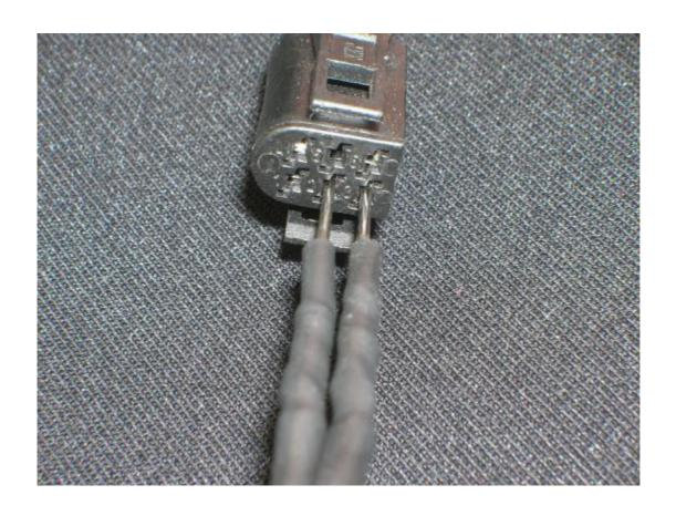
Plug with 6 pins, heads of the cables to pins 2 and 3
