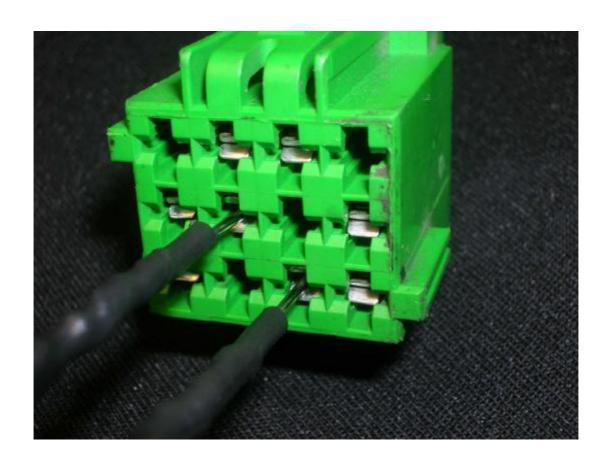
Plug with 12 pins, heads of the cables to pins 6 and 8
