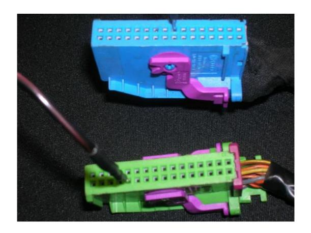
Connect the heads of the cables to 5<sup>th</sup> pin in green plug of instrument cluster and 25<sup>th</sup> in blue plug (in Audi pin 28)
