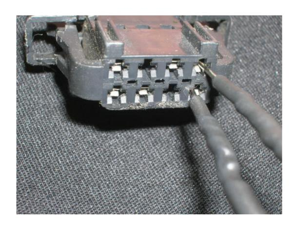
Plug with 8 pins, heads of the cables to pins 7 and 8
