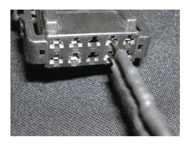
Plug with 10 pins (older cars without CAN) heads of the cables to pins 7 and 8
