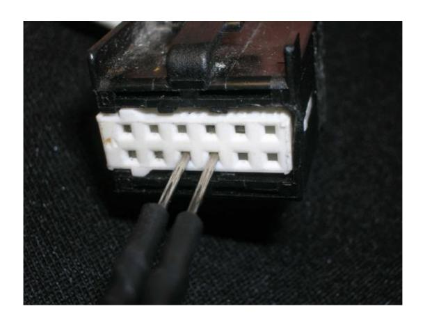
Plug with 12 pins, heads of the cables to pins 9 and 10
